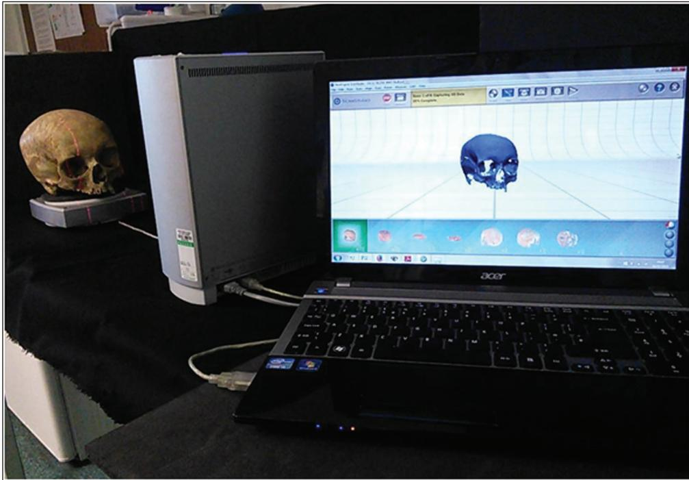
**Figure 1:** NextEngine laser scanner (model 2020i) in use at the Institute of Archaeology, collecting 3D data for a human skull. Photo: Sandra Bond.
