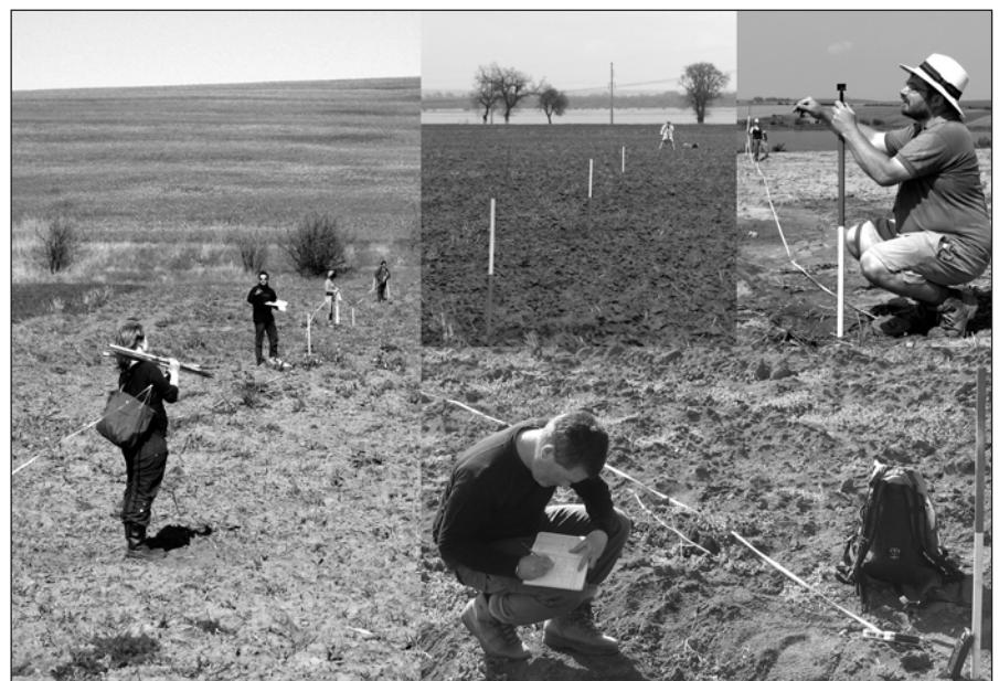
Figure 2 Spot walking at Noviodunum. From top-centre clockwise: laying out the centre line using a total station; setting out the line of spots using an optical right angle; locating the end of a transect using a handheld GPS; a line of spots being walked.
